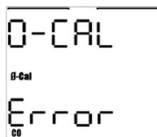
After 3 seconds, the MultiPro will return to the current gas readings screen and the visual and audible alarms will cease.
