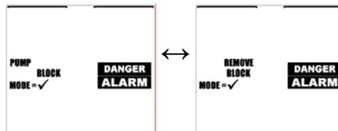
Remove the blockage and press the MODE button to acknowledge the alarm and resume sampling.
