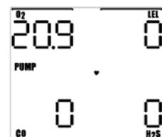
is turned on. If the pump is attached while the instrument is running, the MultiPro will automatically initiate the pump test sequence before returning to the current gas readings screen.
