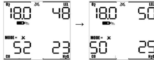
Once the calibration of all sensors is successfully completed, the MultiPro will briefly show the maximum adjustment values screen.
