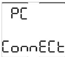
1. With the MultiPro turned off, hold the MODE button down until four beeps are heard. Depending on the software version, this will normally take between 10 and 20 seconds. “PC Connect” will be shown once the infrared port has been activated.
