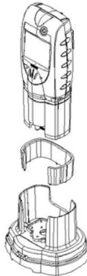
Once the spacer has been inserted, the MultiPro with pump may be charged according to the instruction given in section 5.3.3 above.
