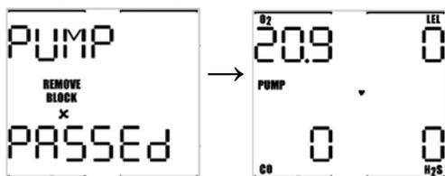
If the instrument is unable to detect the vacuum resulting from the pump blockage within 30 seconds, the test will fail, the instrument will go into alarm and you will be directed to remove the pump.
