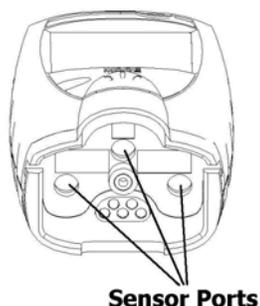
**⚠️WARNING** The sensor ports must be kept free of obstruction. Blocked sensor ports can lead to inaccurate and potentially dangerous readings.
