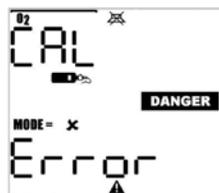
being challenged with calibration gas containing less than 19.0% oxygen, it should be considered out of tolerance and retired from service immediately.
