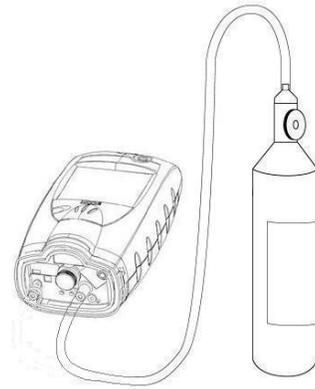
**Figure 4.1 Bump Test / Span Calibration set up**
