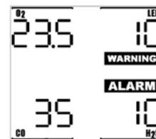
Warning alarms can be temporarily silenced by pressing the MODE button if this option is enabled with BioTrak.
