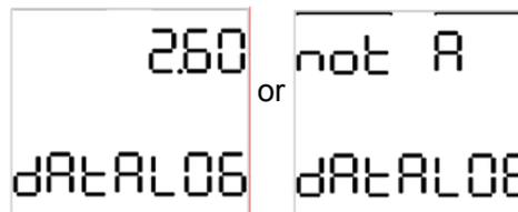
In the MultiPro, the standard one-minute sampling interval will result in the ability to store a minimum of 41 hours of readings before the oldest data is overwritten by new data. The sampling interval may be modified using BioTrak Software.
