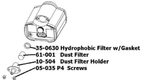
5. Place the new hydrophobic filter with the filter side down in place of the one removed in step 4. The gasket should be located on top of the filter and should sit against the dust filter holder, which will be reinstalled in step 6.
