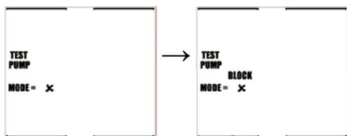
Block the sampling inlet by placing a finger over the end of the sample probe assembly. Once the blockage is detected, the MultiPro will indicate that the test has been passed and instruct you to remove the blockage. Once the blockage is removed, it will proceed to the current gas readings screen.
