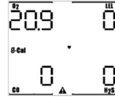
If a successful fresh air / zero calibration is not performed prior to instrument shut down, the MultiPro will show that Fresh Air Calibration is due during instrument start up.
