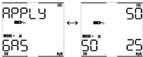
**Note: Sperian Instrumentation recommends the use of multi-component calibration gas for calibrating the MultiPro.**
