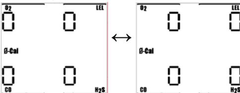
2. The fresh air/zero calibration is complete when the instrument begins another 5-second countdown for the span calibration. If span calibration is not required, allow the countdown to reach 0 without pressing the MODE button.
