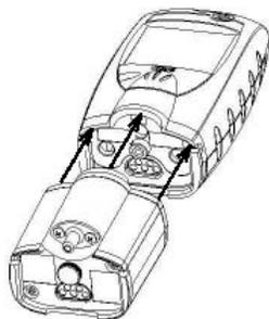
**Note: The sample probe assembly must be attached to the pump when the pump is attached to the instrument.**
