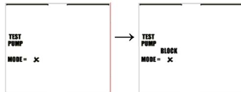
Block the sampling inlet by placing a finger over the end of the sample probe assembly. Once the MultiPro recognizes that the test is passed, it will instruct you to remove the blockage.
