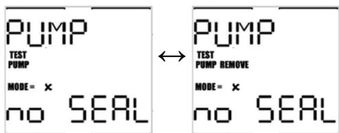
Remove the pump and press the MODE button to resume diffusion operation.
