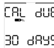
Hold the MODE button down to advance the counter. The number of days shown is the number of days that must pass following a successful calibration before the calibration due warning will be shown. The maximum length of time between calibrations is 180 days.
