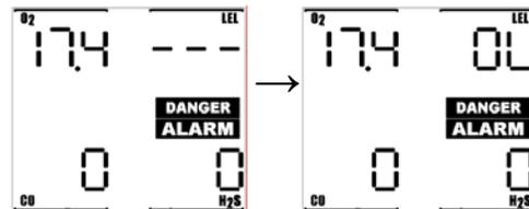
**⚠WARNING** A combustible sensor overrange alarm indicates a potentially explosive atmosphere. Failure to leave the area immediately may result in serious injury or death!
