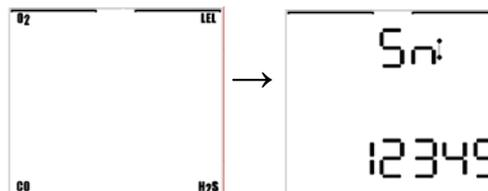
If the MultiPro is equipped with a fully enabled datalogger, the following screen will be shown. The time figure in the upper right corner indicates the sampling interval in minutes and seconds. Instruments without a fully enabled datalogger will show display “not a datalog”
