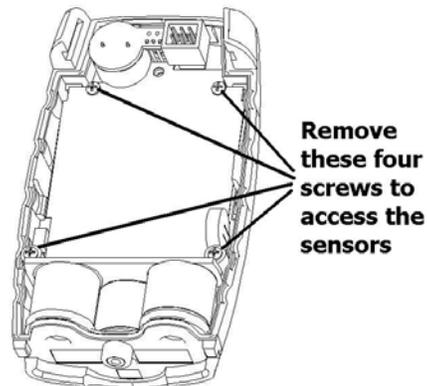
**Note: Sensor channels in the MultiPro are specific to the type of sensor that occupies the channel. When replacing sensors, be sure to replace one sensor with another of the same type.**
